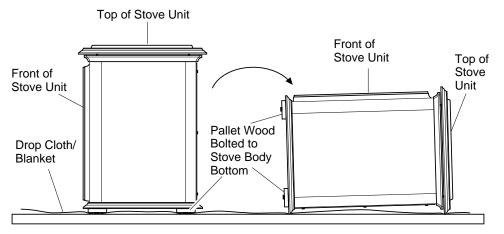
Figure 6 - Laying Down Stove On Back (Stove Style May Vary Depending on Model) Front
